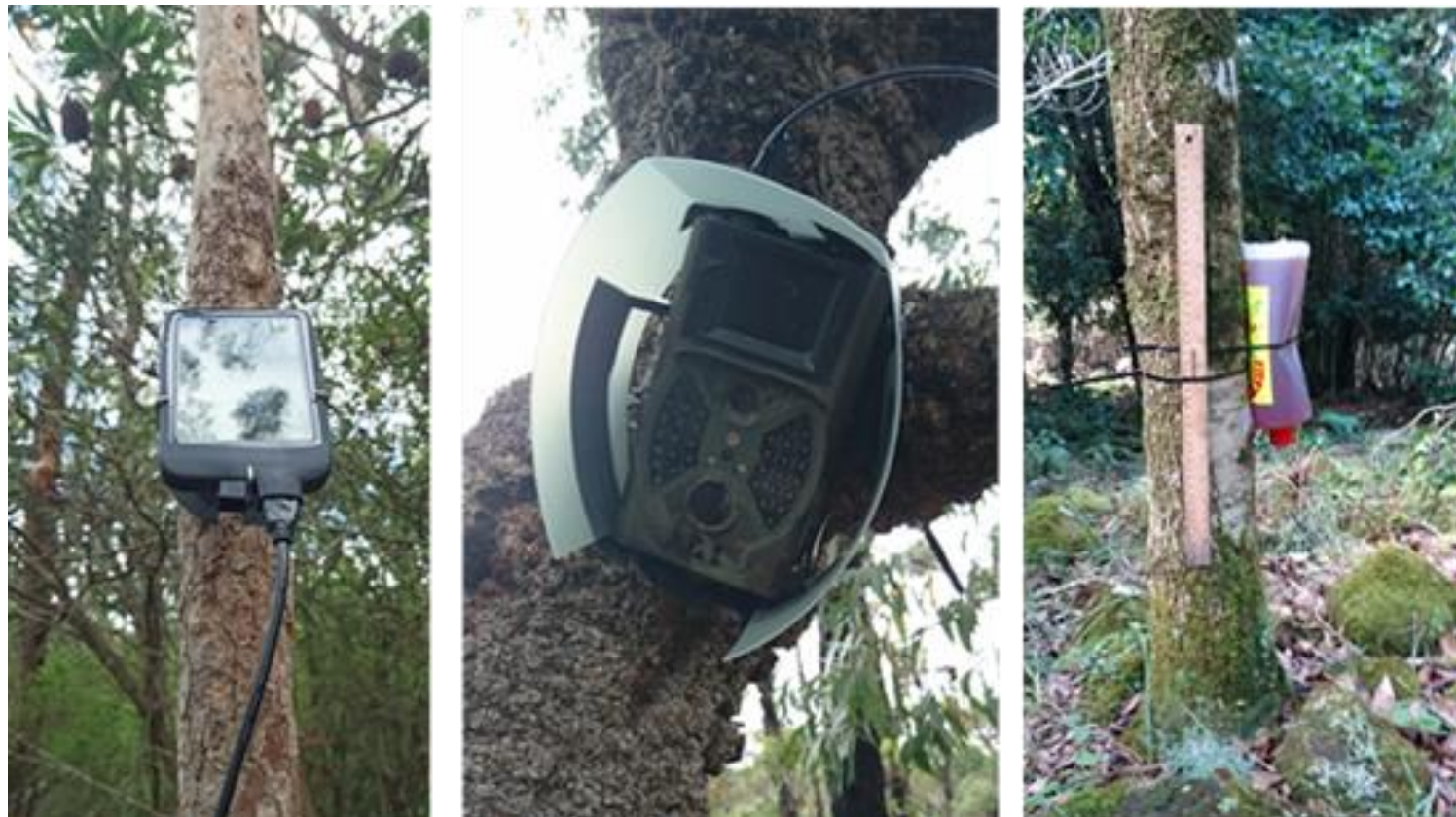
Plate 1. From left to right: Trail camera solar panel, camera with sun and rain shield, long term bait station with inverted bottle of tuna oil and an additional ruler for measurements.
