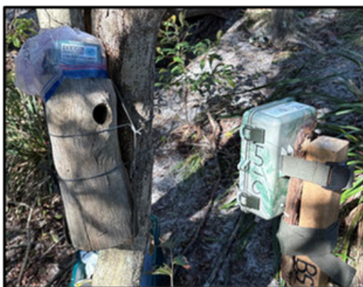
Figure 2. Internal and external cameras, set up with 4x magnification lenses.
