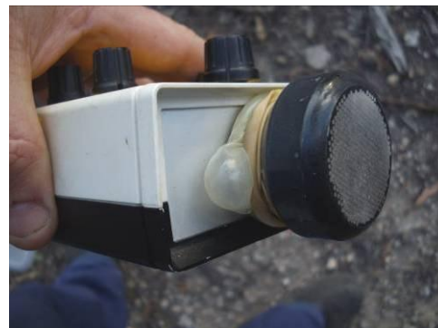
Plate 1: Condom protection on Anabat unit.
