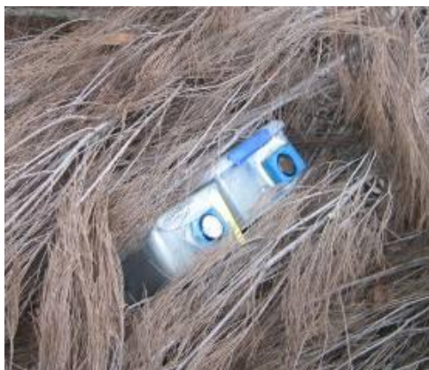
Plate 2: Anabat units in waterproof containers, with sensors exposed.
