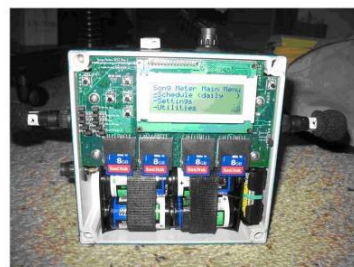
Above: The Wildlife Acoustics Song Meter 2 with microphones attached at sides and cover removed showing internal features (see page 14). Photo courtesy of Paul Burcher
