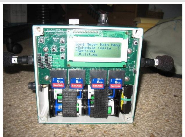
The Wildlife Acoustics SM2 with microphones attached (at sides) and cover removed showing internal features (photo courtesy of Paul Burcher).
